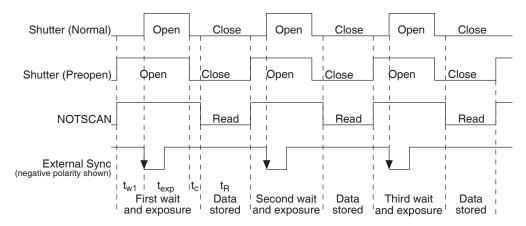
Figure 13. Timing Diagram for the External Sync Mode
